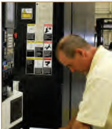
**Marc Rentz can engineer parts using SolidWorks and MasterCam software, and program the most complex CNC machines available. One of these machines is T.R.U.'s Makino A61 Horizontal Machining Center. This machine can constantly run parts without downtime because one work station (called a tombstone) swings into the machine while another tombstone is swung out of the machine to be reloaded with new blanks of material.**
